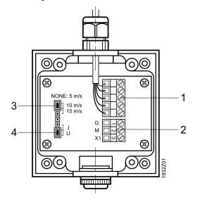
Terminal block for connection to the immersion stem
